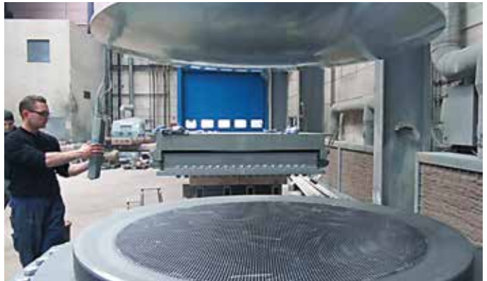
MAURER MSM® Spherical Bearing for 220.000 kN vertical load
