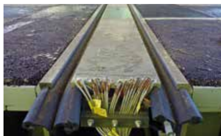
Test setup of intelligent expansion joint for load measurement
