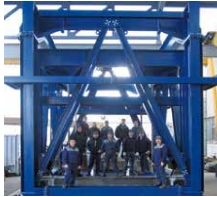
The MAURER factory team illustrates the dimension of the steel frame for the double pendulum of SOCAR Tower in Baku / Azerbaijan
