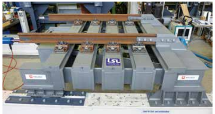
MAURER Guided Cross Tie load test in test lab of Prof. Bucak, Augsburg / Germany
